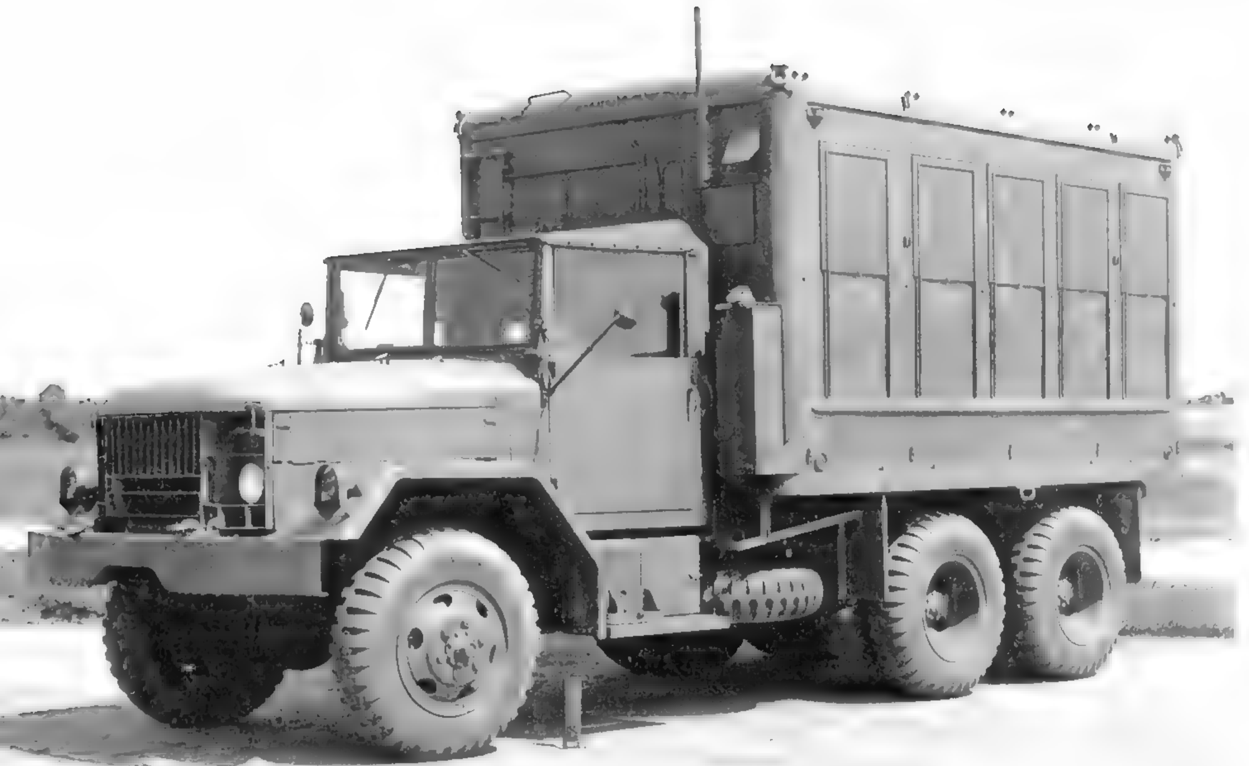
The earliest M109 trucks had five windows per side. In later models, this was reduced to three per side. (National Archives and Records Administration photo)
